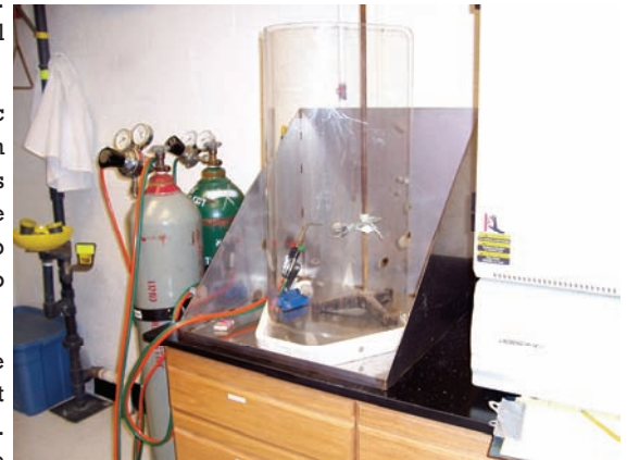
Proper Workstation (Note Shield In Place) and face.
