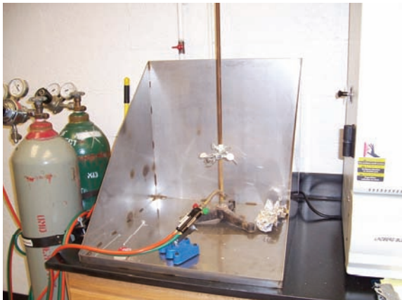
Improper workstation (without shield)
